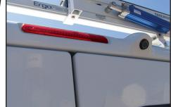
An LED rear brake light is standard, while a rear view camera is an available option.
