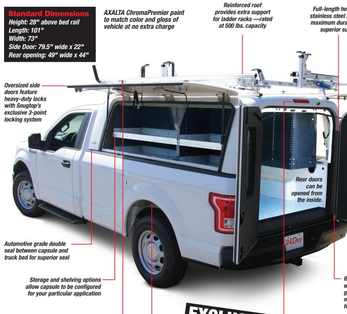
Full-length heavy-duty stainless steel hinges for maximum durability and superior support
